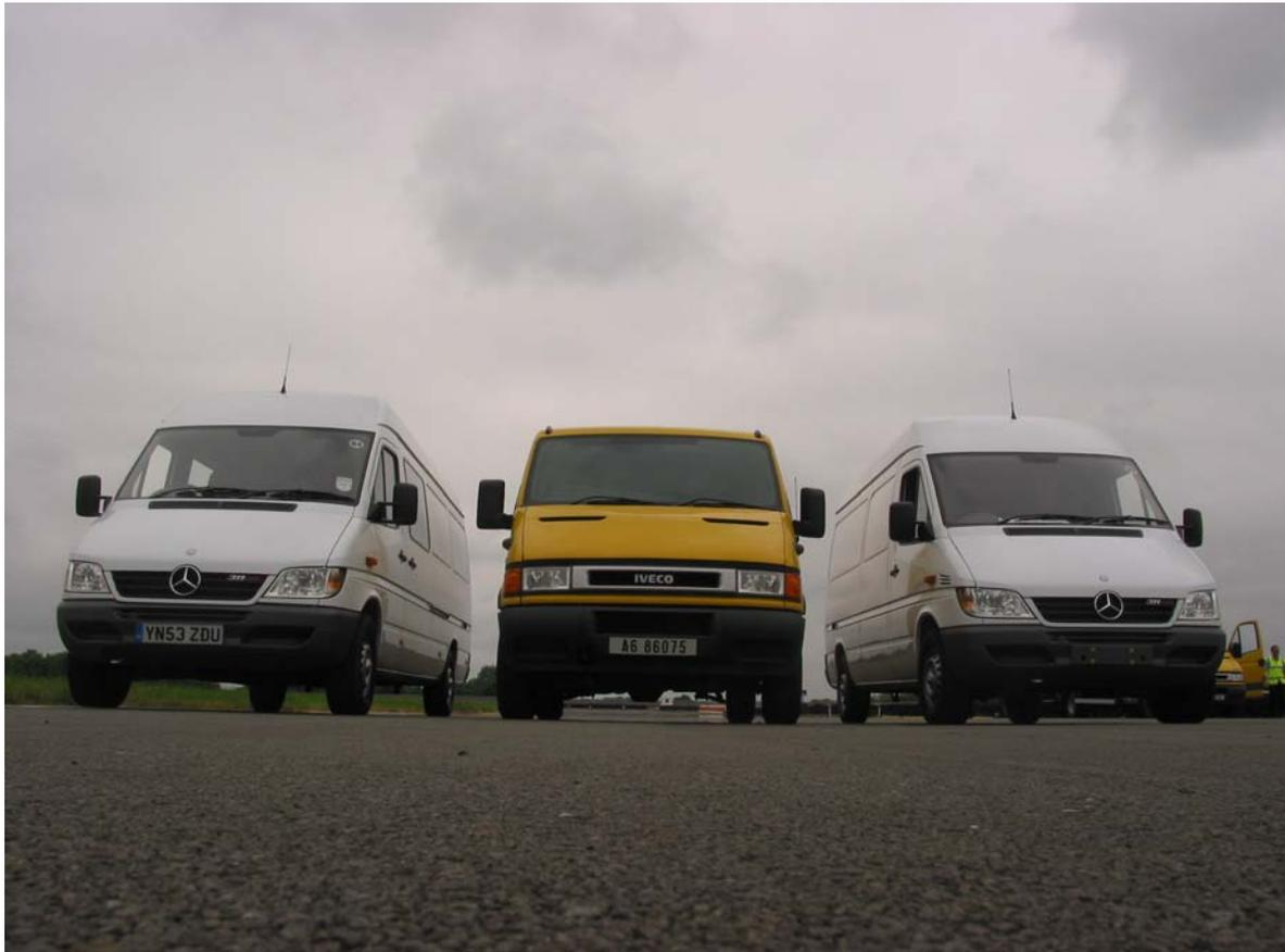
The second pair of vehicles consisted of a Daily 35S12 – 15 and a Sprinter 311CDI – 4250 which were also to complete the standard BTAC test. Unfortunately, during the first part of the tests the driver of the Sprinter did an extra lap at 50 MPH. In order to ensure a valid test the same driver was instructed to complete an extra lap at 50 MPH when driving the Daily. These additional distances were taken into account when calculating the L/100km and MPG shown in Table 8-2.
