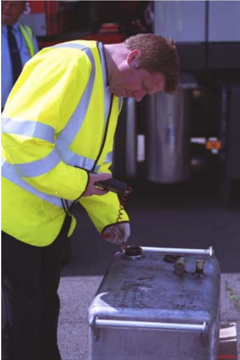
***Check the test fuel temperature***
