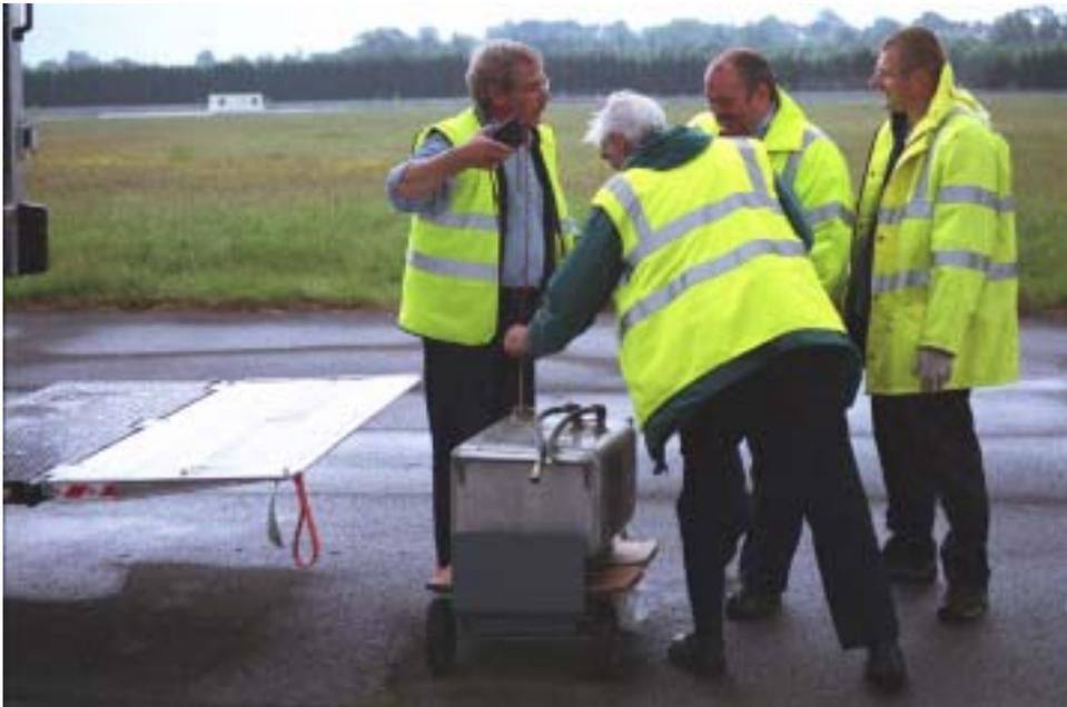
***Test tanks filled with test fuel are weighed prior to test procedure***
