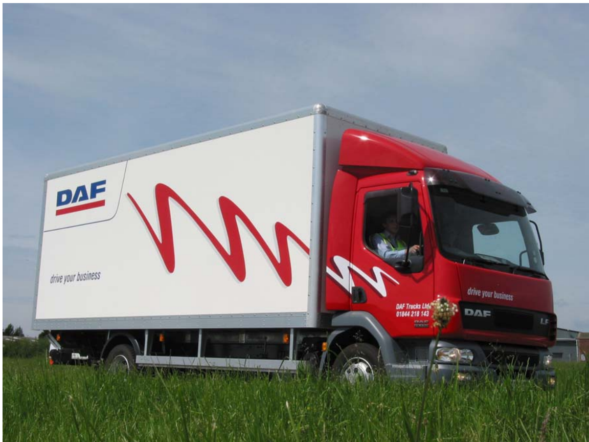
Figure 6-1 7.5 tonne DAF LF 45 almost 17 MPG at 56 MPH.
